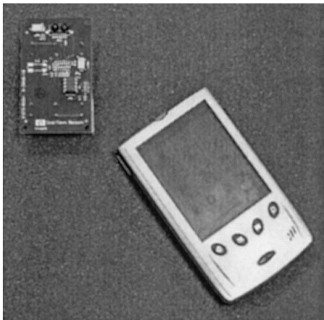
Fig. 1. A palm-sized personal digital assistant (PDA) and an infrared beacon [15]. URL text stored in the beacon can be accepted through the PDA’s infrared port and then used to bring up a location-specific Web page in the PDA’s browser.
