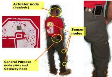
Figure 1. Bio-WWS set up
