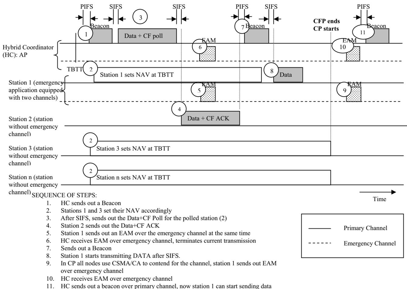
Figure 3: channel access during the Contention Free Period (CFP) and Contention Period (CP)
