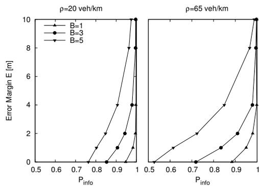
**Figure 6. Required minimum error margin  $E$  [m] as a function of the target probability to inform all nodes in the security area**
