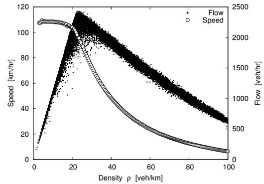
**Figure 2. Vehicular fundamental diagram**
