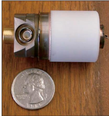
**Carbon nanotube x-ray tube for use in an x-ray diffraction/fluorescence spectrometer. It consists of a film of carbon nanotubes, which emits electrons upon application of an electric field. (figure courtesy of NASA Ames Center for Nanotechnology)**
