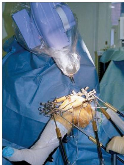
The purple hardware device suspended above the patient's knee is the Acrobot arm. The knee is open for surgery with rods holding it in position. The surgeon's hands [lower right] operate the force control handle during surgery.
