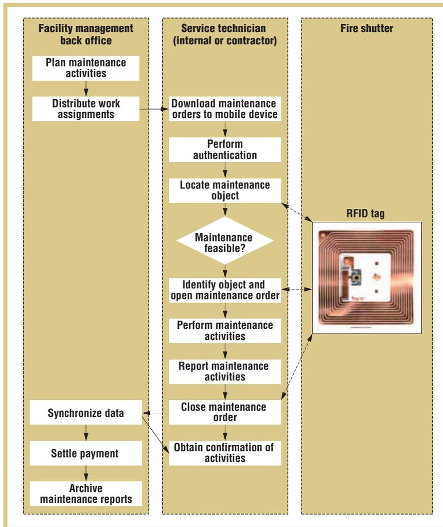
Figure 1. Fraport's new maintenance process.
