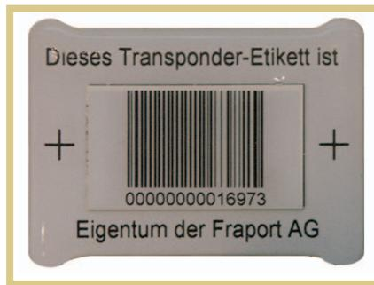
Figure 2. Custom transponder for tagging metallic equipment.
