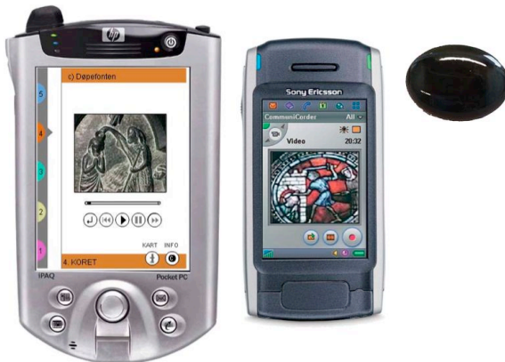
Figure 5. The system running on iPaq and SonyEricsson P900 and the WLAN tag
