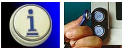
Figure 2. iButton (left) with reader (right).<sup>2</sup>
