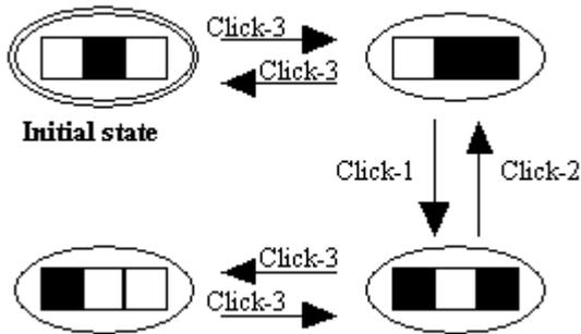
Figure 6. The state transition diagram for an FSA..
