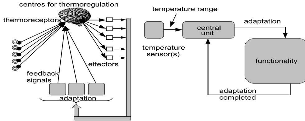
Fig. 2. Global view of the biological system of thermoregulation, left, and the proposed adaptive system, right
