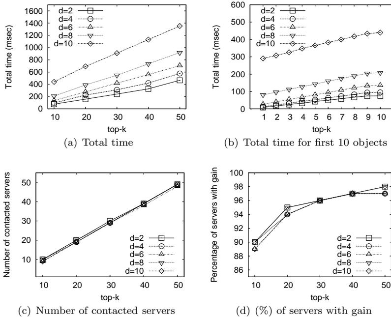
**Fig. 7** Performance (time and contacted servers) of DiTo for varying dimensionality and top- $k$  values
