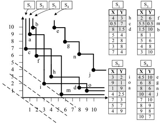
Fig. 4 Example of distributed algorithm for top- $k$  query processing for 4 servers  $S_1, \dots, S_4$ .
