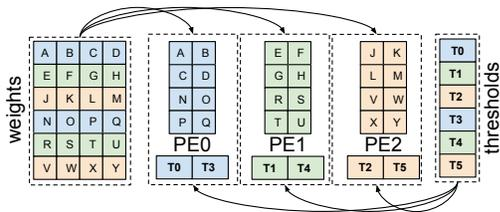
Figure 8: Neuron and synapse folding for MVTU.
