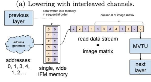
Figure 7: Convolution using interleaved channels.
