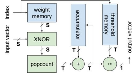
Figure 6: MVTU PE datapath. **Bold** indicates bitwidth.
