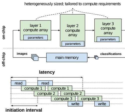
Figure 2: Heterogeneous streaming architecture and schedule.
