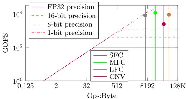
Figure 9: ZC706 roofline with topologies and **max**-datapoints.
