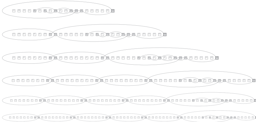
Figure 1-1. An example of the development of a parity circuit. Each line shows the phenotype graph at a given time step. The first graph solves the 2-input parity, the second solves 3-input and continues to 7-bits. The graph has been tested to generalise through to 24 inputs. This pattern of growth is typical of the programs investigated.
