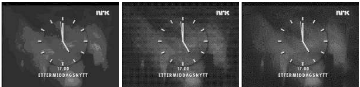
Figure 5.3: No dither to the left, ordered dither in the middle and Floyd-Steinberg dither to the right.
