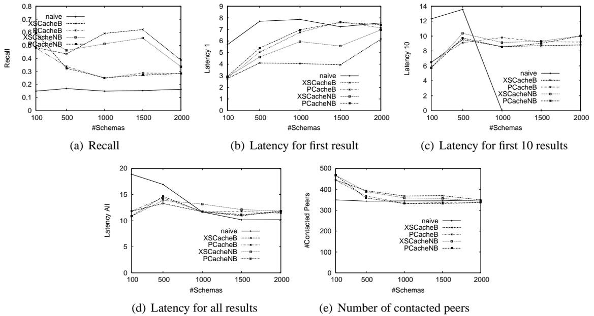
Figure 8: Measurements from using different number of available schemas in the network, employing the GRID topology.
