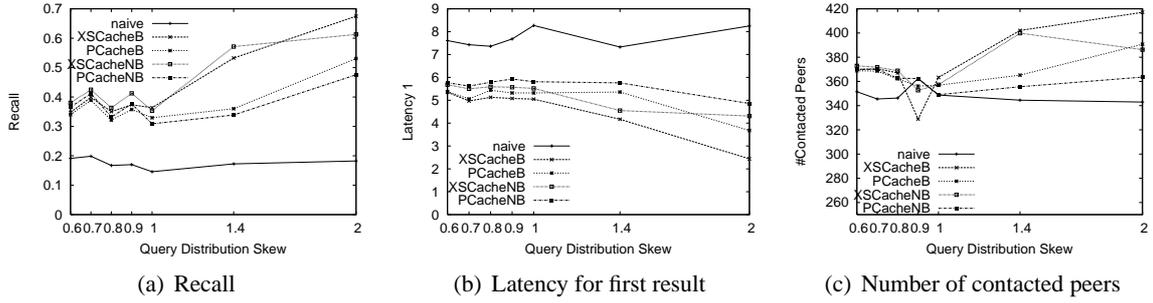
Figure 4: Measurements from using different skew (represented by increasing values of  $a$ ) in the query distributions.
