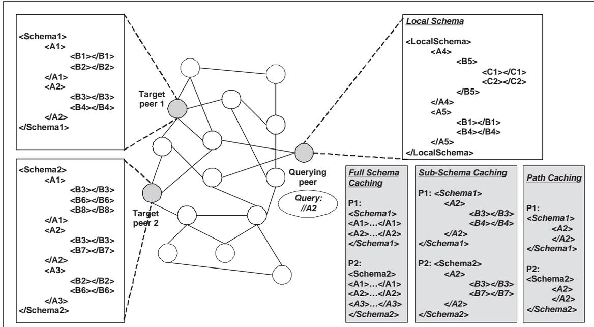
Figure 1: Schema caching variants (*full-schema*, *sub-schema* and *path caching*) as result of a query for `//A2`.
