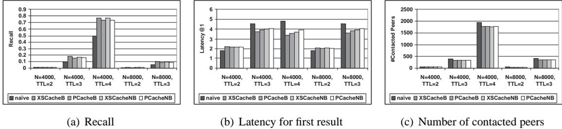
Figure 6: Measurements from using different TTL values in the search, employing GT-ITM topologies of 4000 and 8000 peers and average connectivity degree equal to 7.
