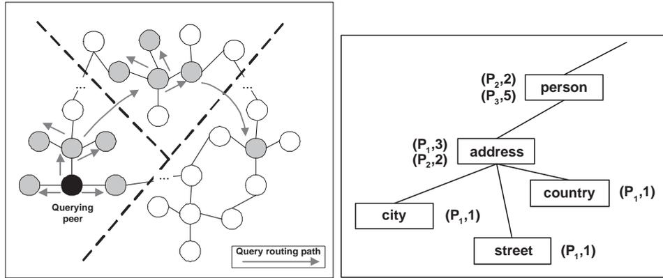
Figure 2: Left: Query routing employing jumps (dashed lines show remote parts of the P2P network, while grey-colored peers are the ones contacted by the query). Right: Tree representation of (parts of) schemas cached from different peers.
